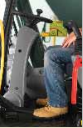
• Steering column pivots for visibility and comfort.
