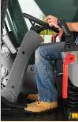
• Steering column pivots for visibility and comfort.
