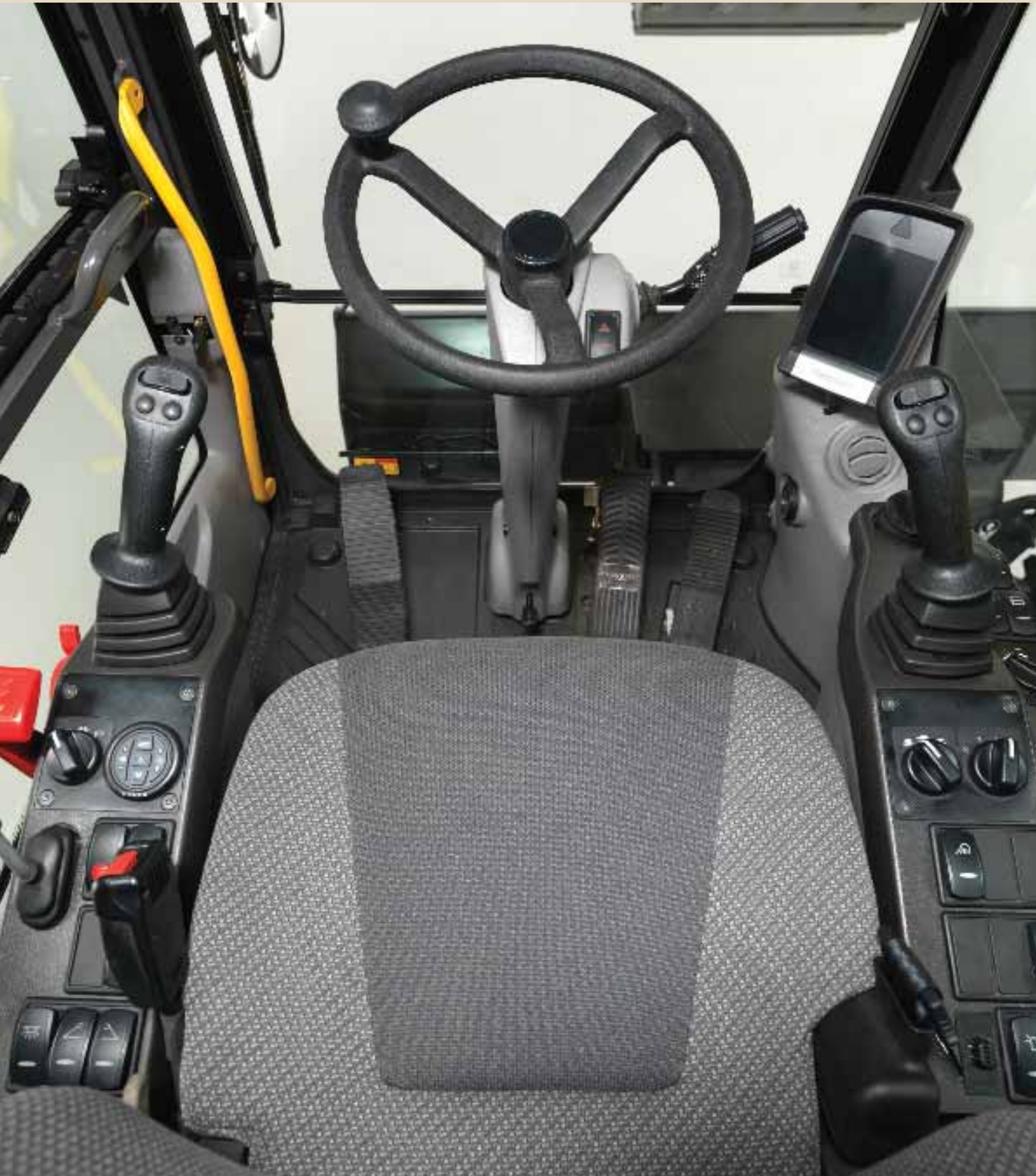
• Steering column pivots for visibility and comfort.
